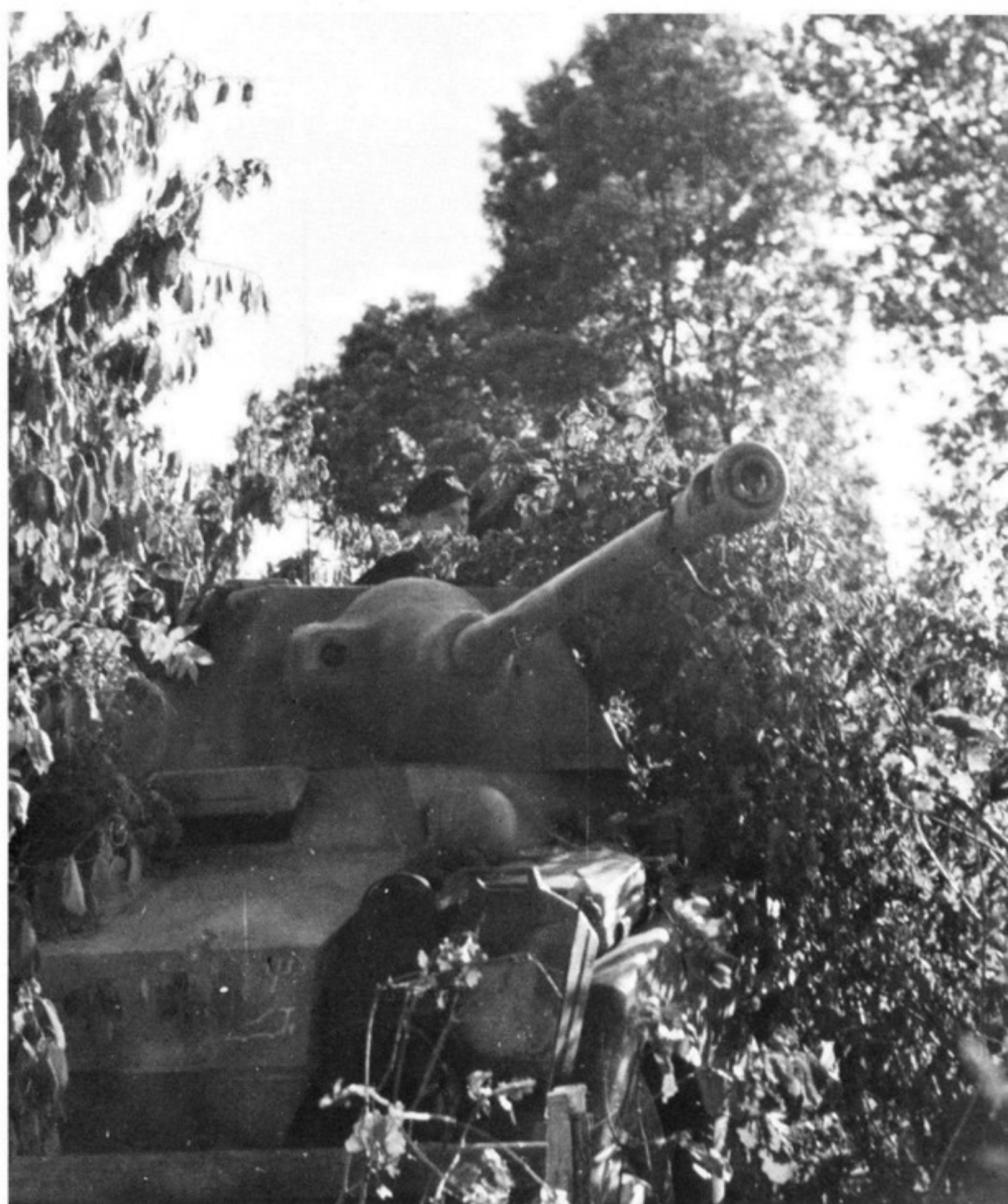
A front view of a PzKpfw IV ausf H shows standard markings, all in white: the trident, vehicle chassis number, and outlined turret numbers. Many 2. PD tanks carried all these markings. (Bundesarchiv)
